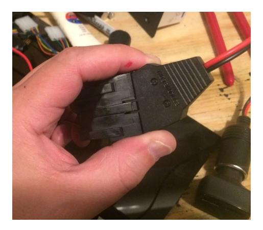
If the connector will not go in easily, the plug can be unclipped from the glovebox to let you use 2 hands to push the ends together. The connector is simply clipped to the side of the glove box. Looking underneath it will show you the wire and plug.
