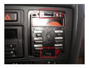
4) Pull OBC gently towards you, flip up the black lever & remove the female wiring connector from the back of the OBC. It will have 12 female connector openings. Your adapter posts will plug into this. For the sake of this guide, the top part we'll call the 'wire side' and the other the 'bottom side'
